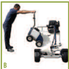
B Raise rear of the Kombi and rotate clockwise.
